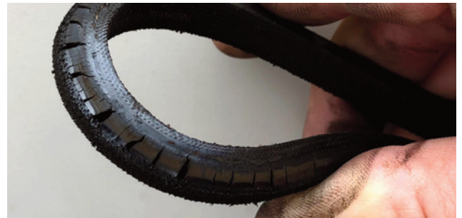
Figure 77. Worn fan belt
