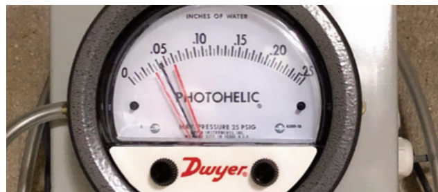
Figure 74. Dial meters can measure both positive and negative pressure
