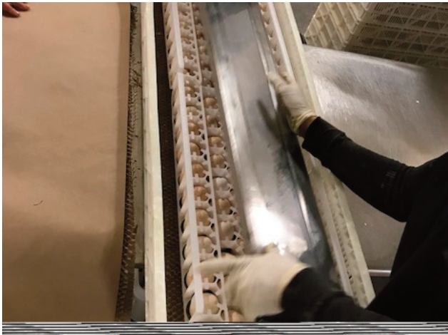
Figure 40. A hatcher basket is then placed on top of the eggs, flats, and slide. The entire basket and eggs are then inverted
