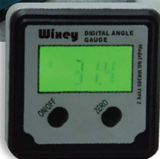
Figure 21a. Angle meter Figure 21b. Digital angle gauge. In both pictures the turning angle is too low, at around 30 degrees
